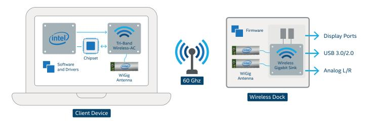
**Figure 1.** Intel Wireless Docking: Every component, from drivers and firmware to the silicon Tri-Band Wireless-AC module, antennas and dock "sink" chip, are developed and tested together to provide the best solution for the end-user.
